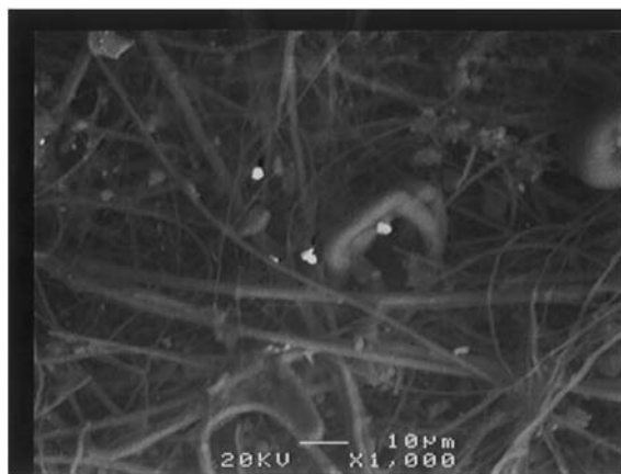
Fig. 3. Image of scanning electron microscopy for sample F16, showing gold flakes (light spots) of different sizes.
